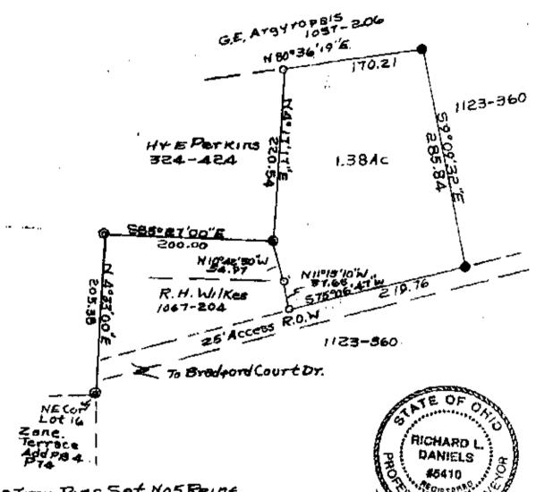
•Iron Pins Set No5 Reinf Bar 30" Lg Plastic IDCap © Iron Pipe Found o Iron Pins Found
