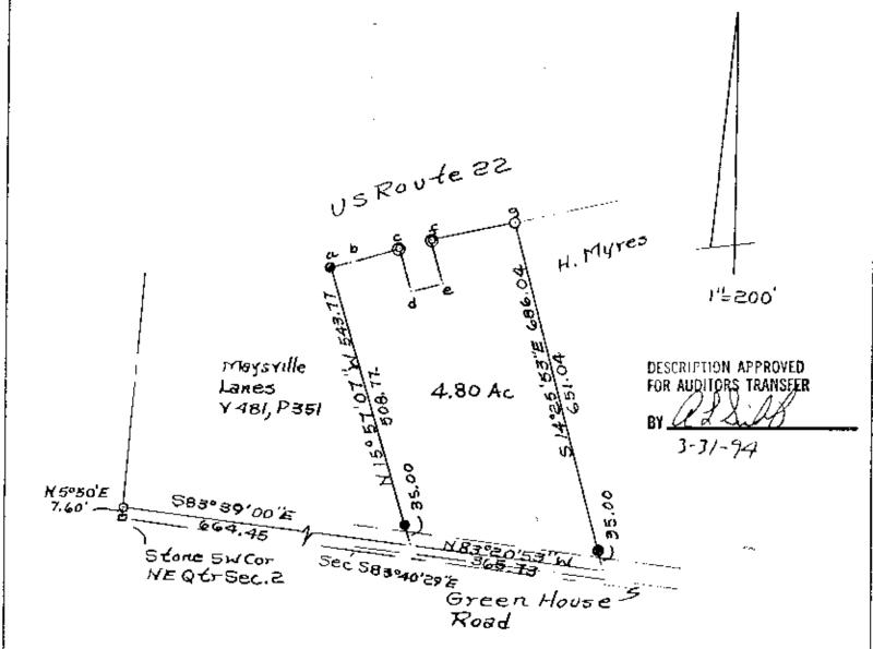
0-b N74°04'07"E 36.36 b-C N75°34'07"E 96.40 C-d S14°26'39"E 78.65 d-e N75°05'11"E 59.88 e-f N14°21'39"W 88.09 f-g N75°34'07"E 162.93
