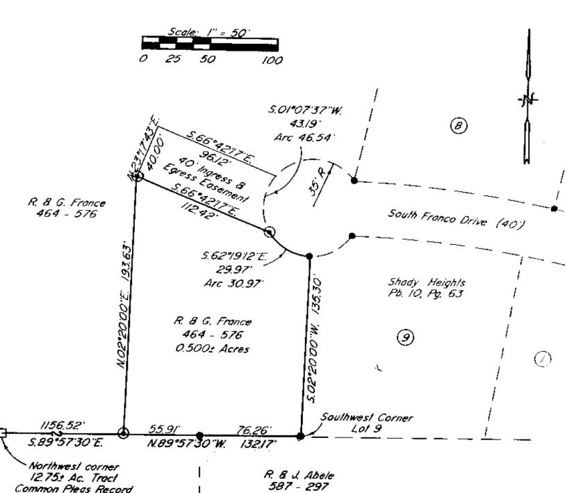
Bearings are based on the Plat Bearings of Shady Heights ( Pb. 10, Pg. 63 ).
