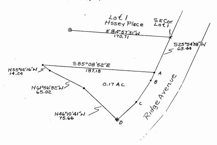
A-B S 26°10'29"W 13.13 B-C S 35°07'22"W 42.70 C-D S 48°39'04'W 43.31 × Hole Drilled In Walk Found
