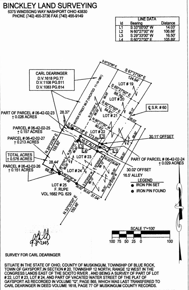
BASIS OF BEARING: BEARINGS ON THIS PLAT ARE ASSUMED ON THE CENTERLINE OF S.R. # 60 AS BEING N33^00'00" E AND ARE FOR ANGULAR CALCULATION ONLY.
