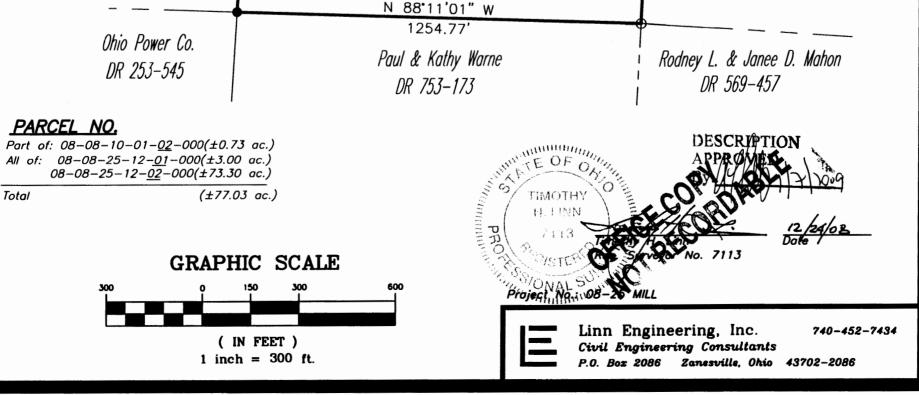
Bearings are based on the Ohio State Plane Coordinate System, South Zone, NAD83 per GPS Observation on 11/01/08.
