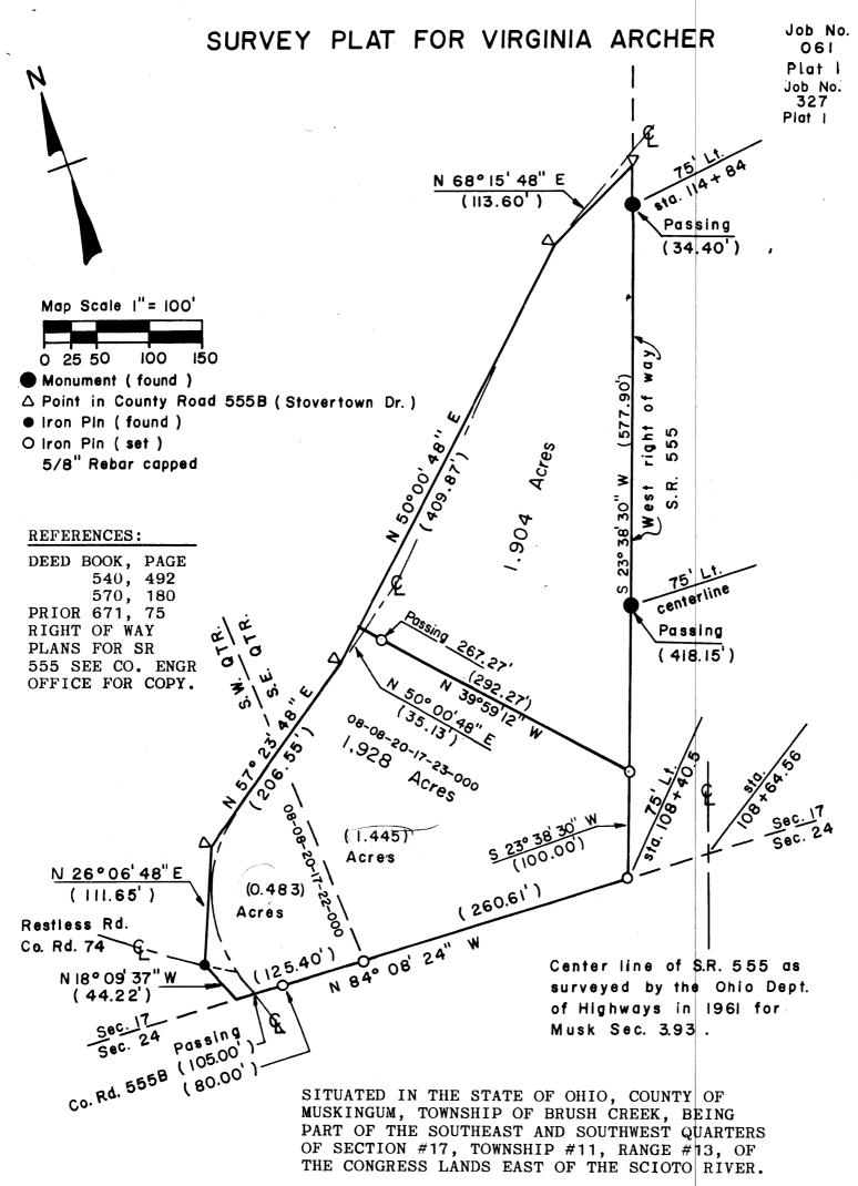
THE BEARINGS, SAID RIGHT OF WAYS, AND THE SOUTH LINE OF SAID SECTION #17 ARE BASED ON RIGHT OF WAY MONUMENTS FOUND AT 75 FEET LEFT OF STA. 114+84, 75 FEET LEFT OF STA. 111+00.25, AND 75 FEET RIGHT OF STA. 110+30 ALL OF SAID CENTER LINE SURVEY.
