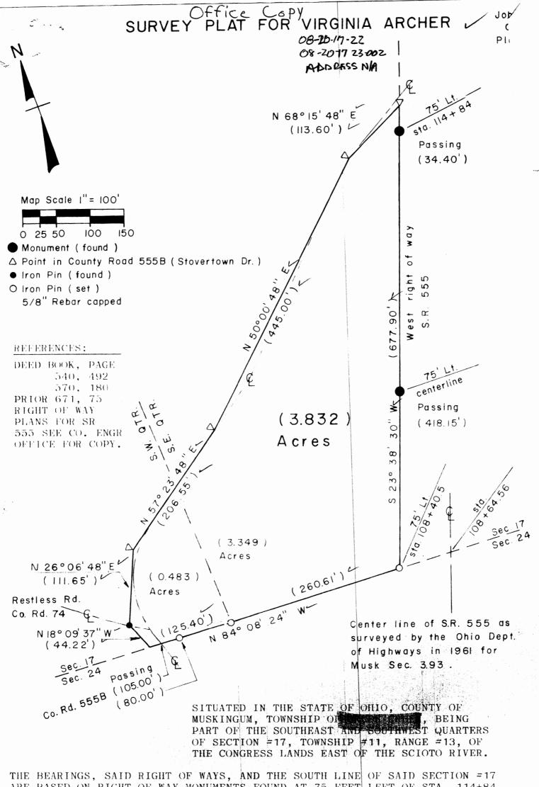
THE BEARINGS, SAID RIGHT OF WAYS, AND THE SOUTH LINE OF SAID SECTION =17 ARE BASED ON RIGHT OF WAY MONUMENTS FOUND AT 75 FEET LEFT OF STA. 114+84 75 FEET LEFT OF STA. 111+00.25, AND 75 FEET RIGHT OF STA. 110+30 ALL OF SAID CENTER LINE SURVEY.
