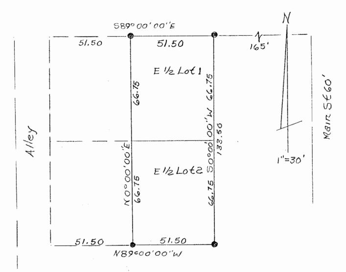
Iron Pins Set No. 5 Reinf Bars 30"Lg Plastic I.D. Čaps
