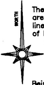
The bearings on this plat are based on the South line of Orchard Hill Road, of Home Acres, being S 85°10'00"E.
