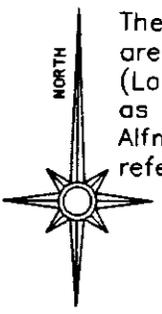
The bearings within the description are based on a Solar Observation (Local Hour Angle Method) completed as part of the survey for the Gerald Alfman property as described in deed reference Volume 1025, Page 411.
