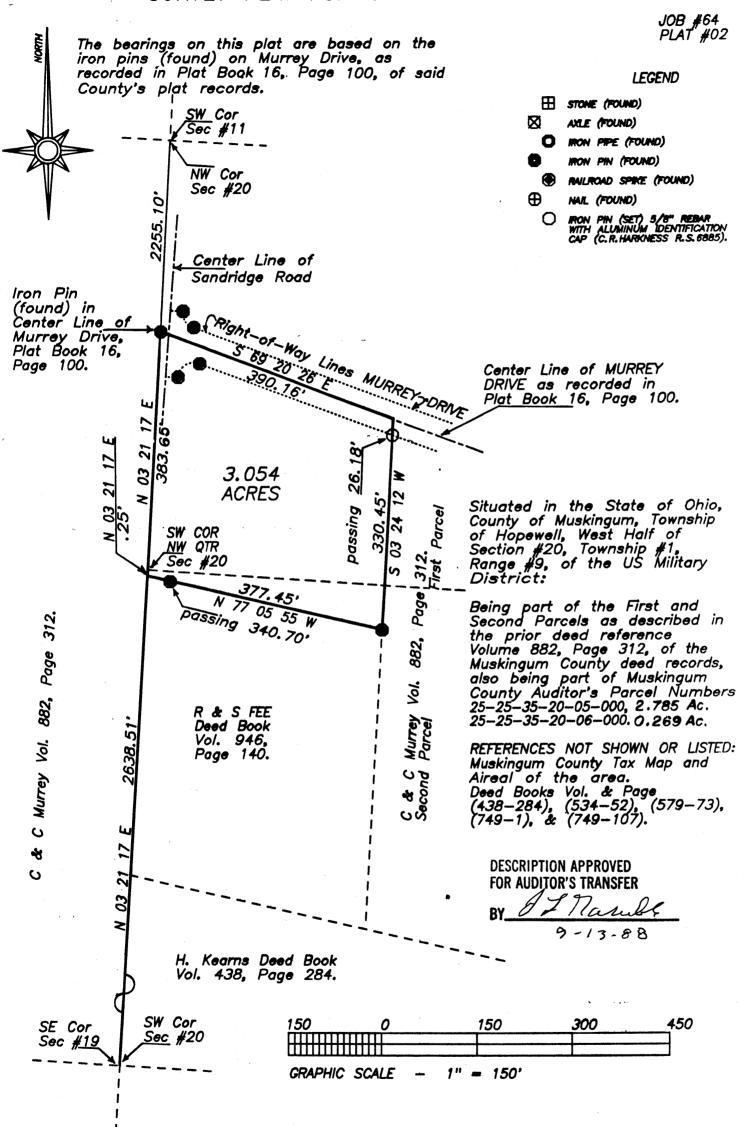
This survey plat was prepared by Charles R. Harkness Registered Surveyor #6885 from an actual survey completed September 2, 1988, and is intended to be used for the legal transfer of the property shown, and does not intend to shown all or any easements of record, nor encroachments unless otherwise indicated.
