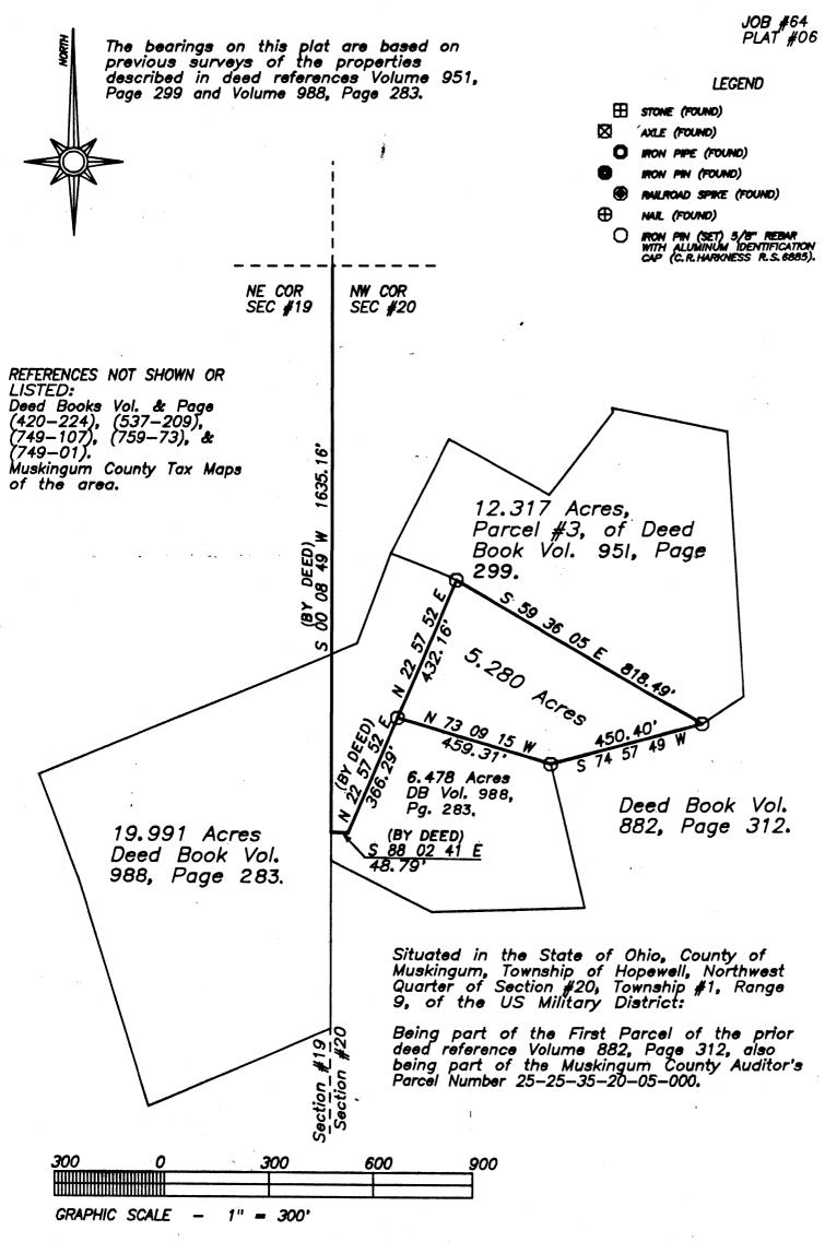
This survey plat was prepared by Charles R. Harkness Registered Surveyor #6885 from previous surveys, the lasOFFICE COPY completed on April 24, 1986, and is intended to be used for the legal transfer of the property shown, and does not intend to show all or any easements of record, nor encroachments unless otherwise indicated.
