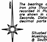
The bearings on this plat are based on the iron pins (found) on Murrey Drive as recorded in Plat Book #16, Page #100, and are shown in a format of Degrees, Minutes & Seconds. Distances are shown in feet and decimal parts thereof.
