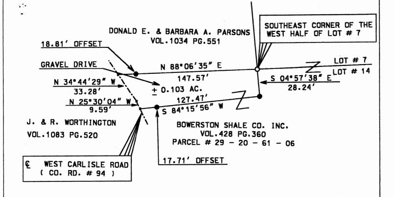
BASIS OF BEARING: BEARINGS ON THIS PLAT ARE ASSUMED ON THE SOUTH LINE OF LOT # 7 AS BEING N 88°06'35" E AND ARE FOR ANGULAR CALCATION ONLY.
