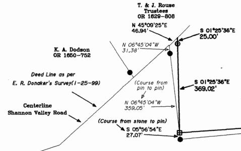
NOTE: Stone found approximately 4 inches by 12 inches, with the top damaged from farm equipment and leaning toward the north. I straightened the stone to a vertical center to reference my survey. This stone was called for in the original deed of Hilty's land.
