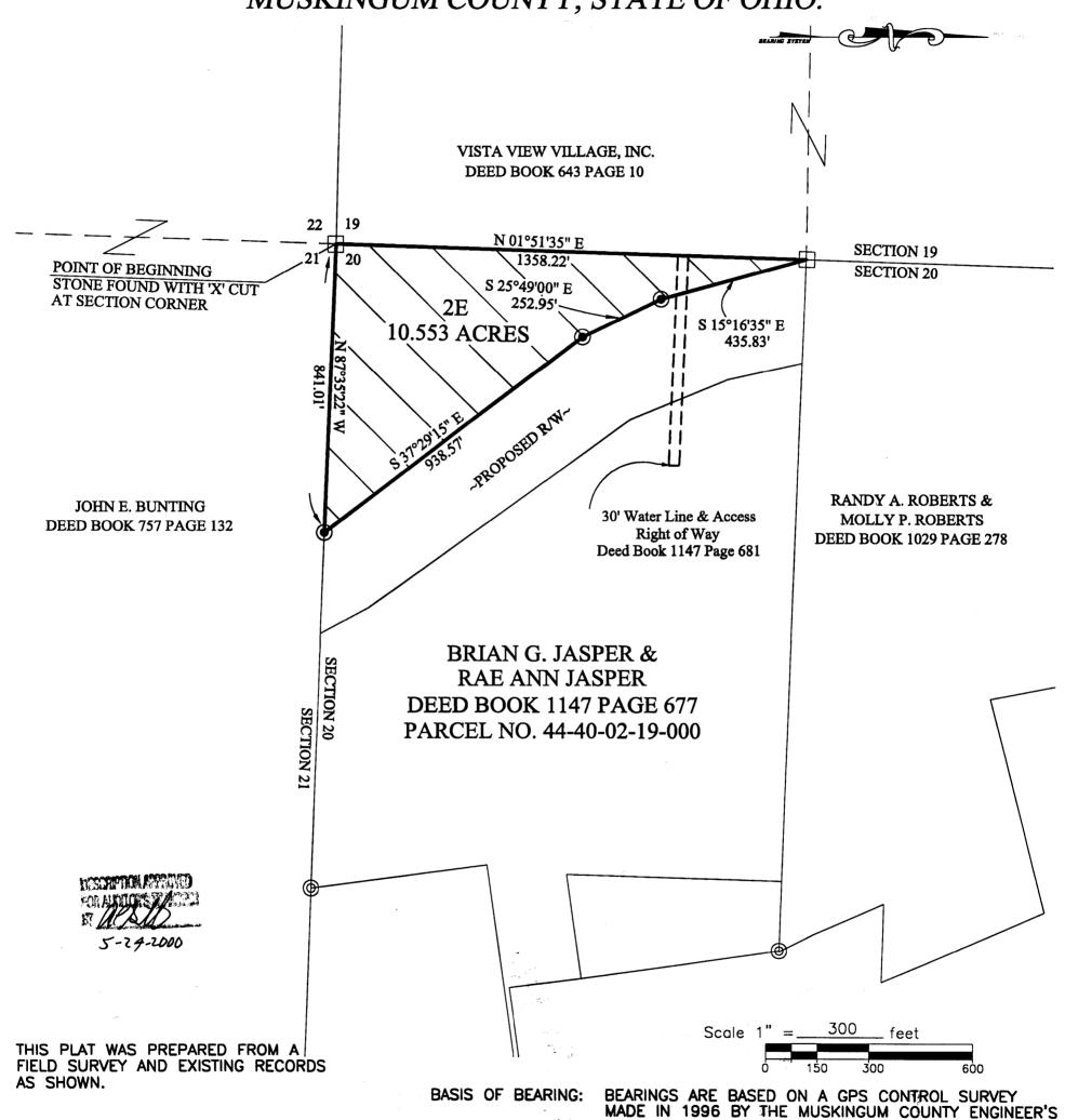
BEARINGS ARE BASED ON A GPS CONTROL SURVEY MADE IN 1996 BY THE MUSKINGUM COUNTY ENGINEER'S OFFICE AND ARE FOR PROJECT USE ONLY.
