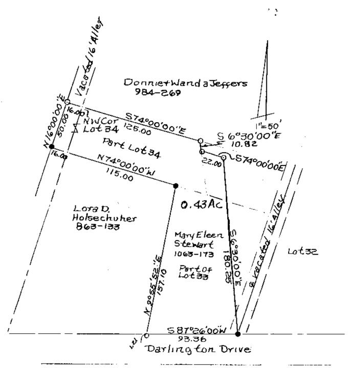
o Iron Pins Found • Iron Pins Set No.5 Reing Bars 30" Lg Plastic I.D.Caps
