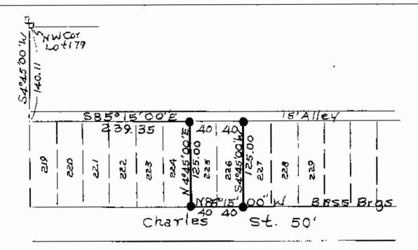
o Stone Found O I ron Pins Set 56 Reinf. Bar. 30"Lg Plastic ID Cap
