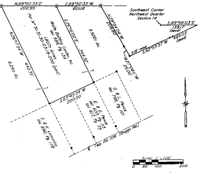
Bearings are based on an assumed bearing of N.89°50'33'E. assigned to the North Line of the said 34 Quarter of Township I, Range 6.
