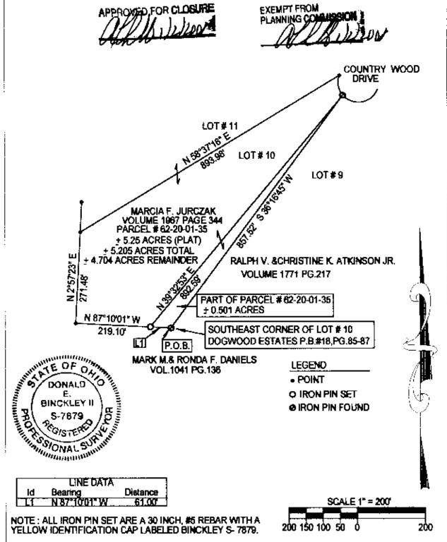
BASIS OF BEARING : BEARINGS ON THIS PLAT ARE ASSUMED ON THE EAST LINE OF LOT # 10 OF DOGWOOD ESTATES AS BEING S 36 DEGREES16 MINUTES 45 SECONDS WEST, AND ARE FOR ANGULAR CALCULATION ONLY.
