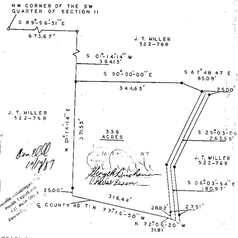
BEARINGS ARE BASED ON THE . WEST LINE OF SECTION. II AS BEING N OO° 56-38"W
