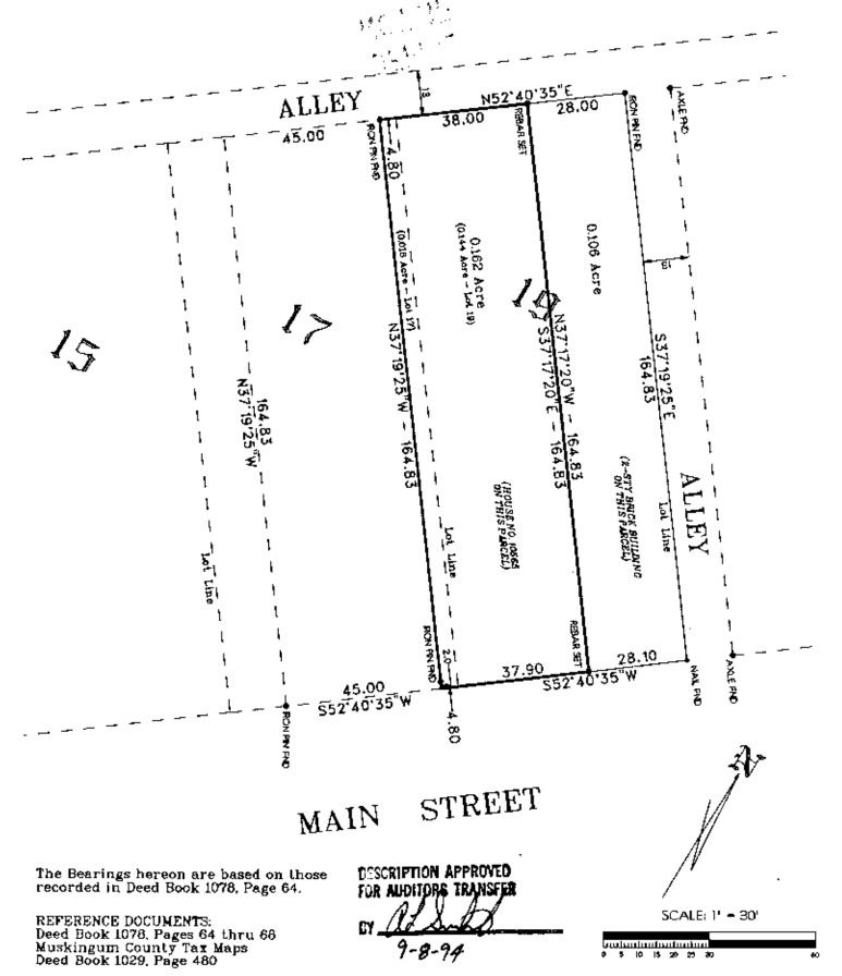
Iron Pins (rebar) set are 1/2 inch diameter and 30" long.
