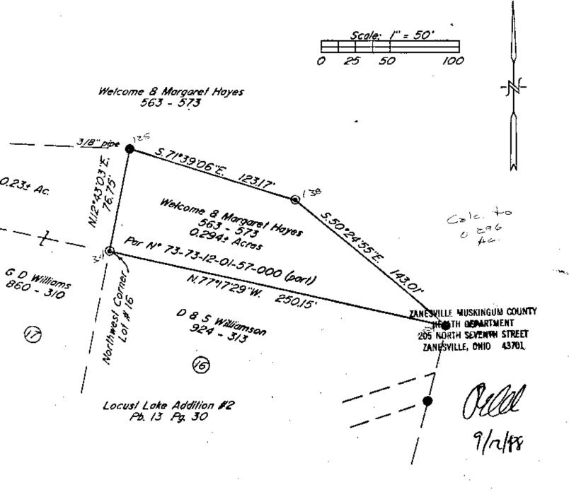
Bearings are based on the plat bearing of the West Line of Lot 28 of Locust Lake Addition #2 ( Pb. 13 Pg. 30 ).
