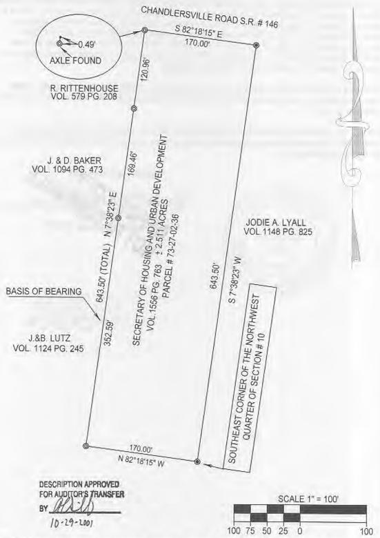
BASIS OF BEARING: BEARINGS ON THIS PLAT ARE ASSUMED ON THE EAST LINE OF A SURVEY BY TERRY FINLEY OF THE TRACT RECORDED IN DEED VOLUME 518, PG.500 AS BEING N 07\*38'23" E AND ARE ASSUMED FOR ANGULAR CALCULATION ONLY.
