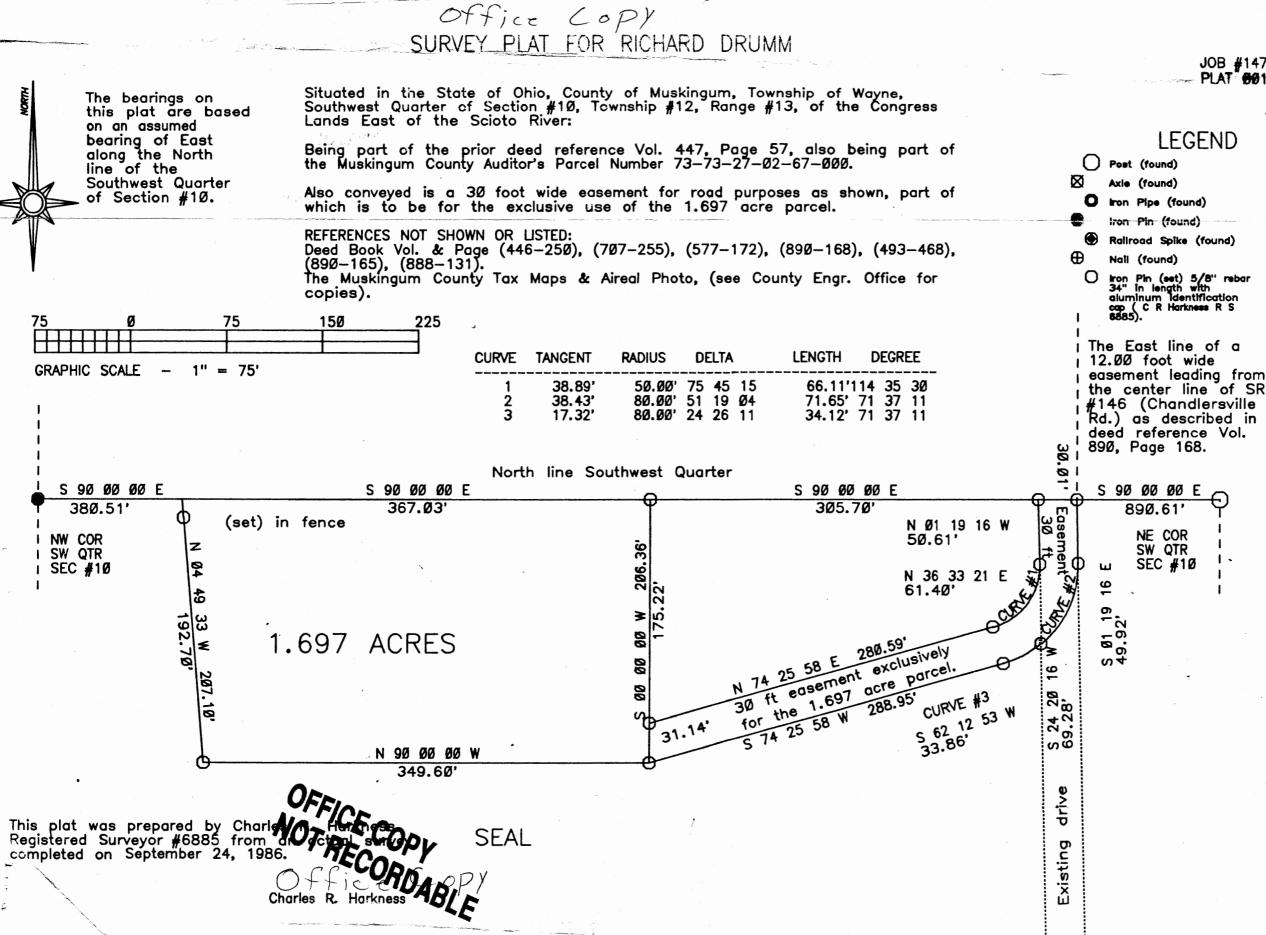
JOB #147 PLAT #01 LEGEND iron Pin (set) 5/8" rebar 34" in length with aluminum identification cap ( C R Harkness R S 6585). easement leading from
