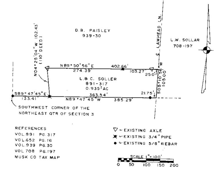
BEARINGS ARE BASED ON THE WEST LINE OF A TRACT CONVEYED TO P.B.C. HAYES IN VOL.652 PG. 16.
