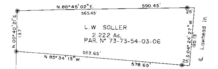
Bearings are based on the west line of a tract conveyed to P.& C. Hayes in D.B. Vol. 652 Pg. 16
