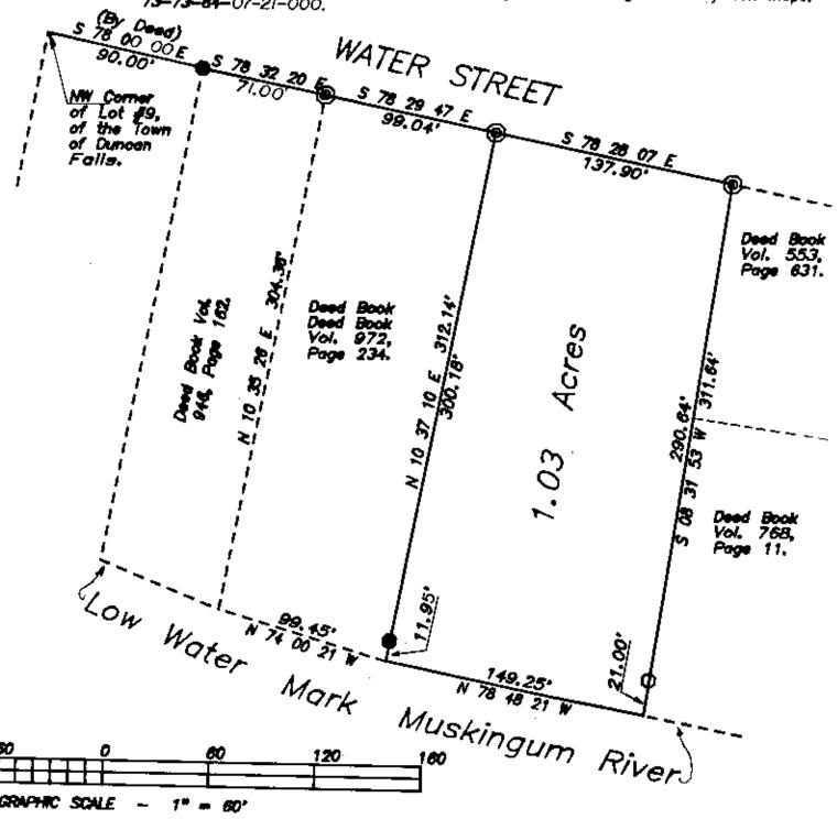
This survey plot was prepared by Charles R. Harkness Registered Surveyor \$6885 from on actual survey completed May 25, 1990, and is intended to be used for the legal transfer of the property shown, and does not intend to show all or any easements of record, nor encroachments unless otherwise indicated.
