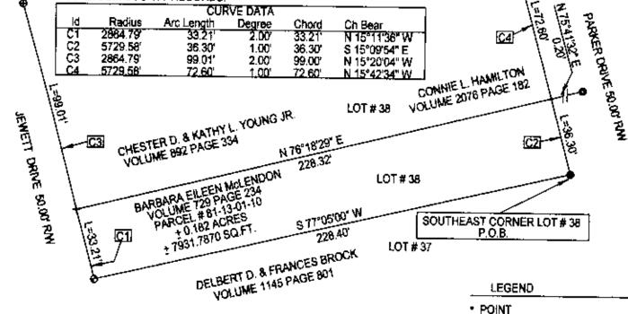
BASIS OF BEARING: BEARINGS ON THIS PLAT ARE ASSUMED ON THIS SOUTH LINE OF LOT # 38. AS BEING SOUTH 77 DEGREES 05 MINUTES 00 SECONDS WEST AND ARE FOR ANGULAR CALCULATION ONLY.
