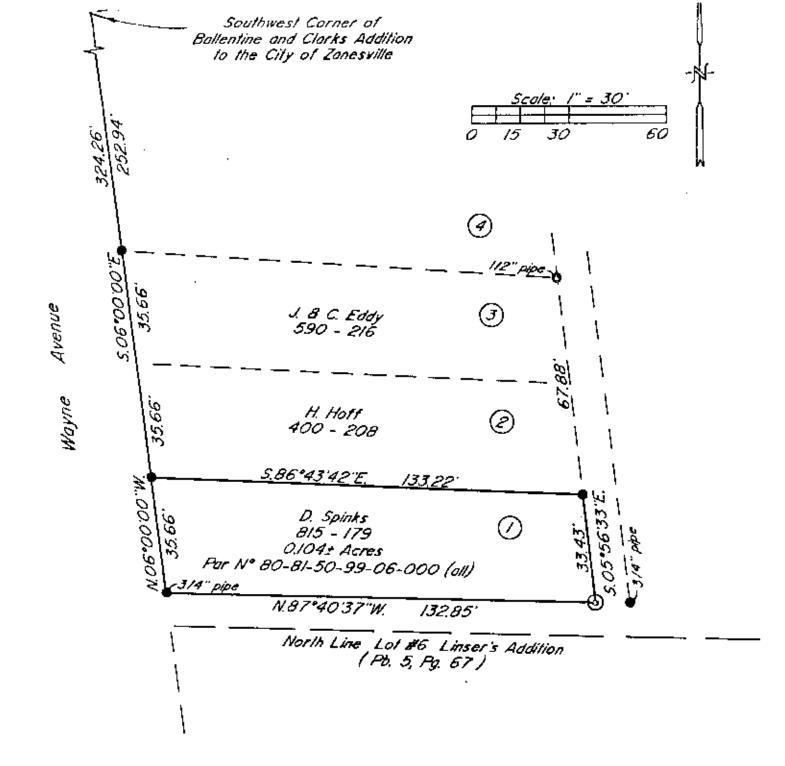
Bearings are based on Deed Bearing of the East Line of Wayne Avenue ( Vol. 590, Pg. 216 )
