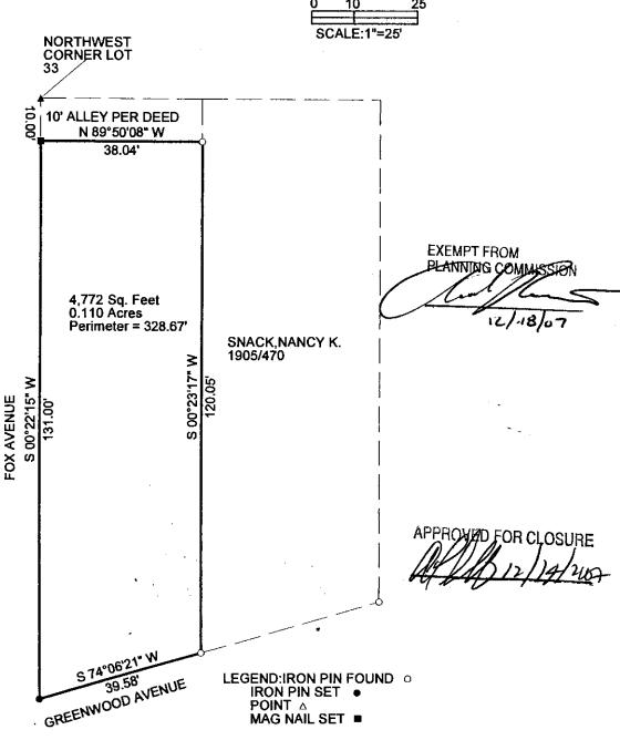
THE BEARINGS SHOWN HEREON ARE BASED ON THE WEST LINE OF LOT #33 AS S-00-22-15-W.
