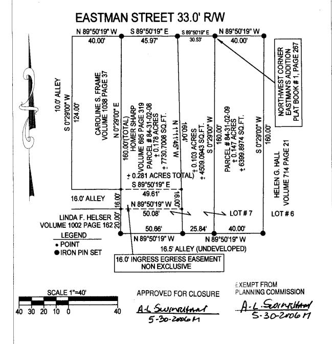
BASIS OF BEARING: BEARINGS ON THIS PLAT ARE ASSUMED ON THE SOUTH RIGHT OF WAY LINE OF EASTMAN STREET AS BEING SOUTH 89 DEGREES 50 MINUTES 19 SECONDS WEST AND ARE FOR ANGULAR CALCULATION ONLY.
