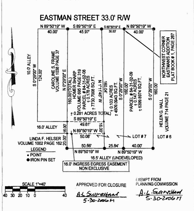
BASIS OF BEARING: BEARINGS ON THIS PLAT ARE ASSUMED ON THE SOUTH RIGHT OF WAY LINE OF EASTMAN STREET AS BEING SOUTH 89 DEGREES 50 MINUTES 19 SECONDS WEST AND ARE FOR ANGULAR CALCULATION ONLY.
