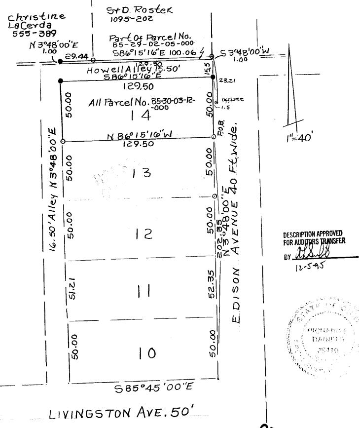
o Iron Pins Found ● Iron Pins Set No 5 Reinf Bar 30"Lg. Plastic ID Cap Linde Hart Lee Jay
