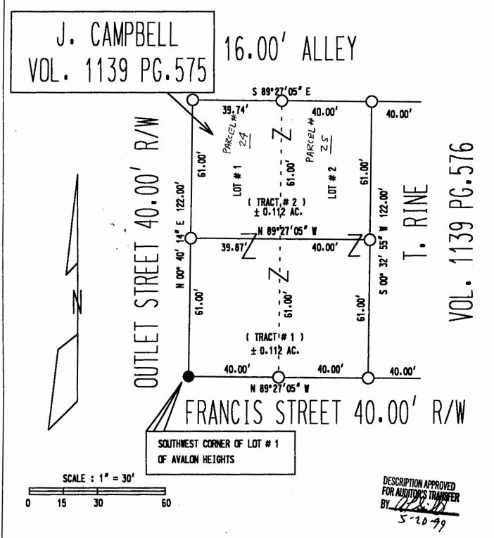
BASIS OF BEARING : BEARINGS ARE ASSUMED ON THE WEST R/W LINE LONG STREET AS BEING S 00° 32' 55" W AND ARE FOR ANGULAR CALCULATION ONLY .
