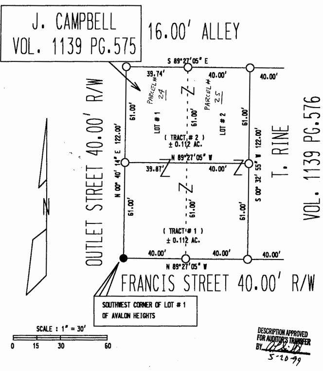
BASIS OF BEARING: BEARINGS ARE ASSUMED ON THE WEST R/W LINE LONG STREET AS BEING S OO° 32' 55" W AND ARE FOR ANGULAR CALCULATION ONLY.
